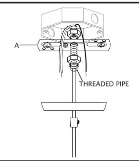
10. Slightly loosen ground screw on mounting bracket (A). Do not completely remove ground screw. Wrap house ground wire (copper) around ground screw, leaving enough ground wire to attach to fixture ground wire. Twist end of fixture ground wire and end of house ground wire (copper) together. Twist wire connector (C) onto ends of wires. Completely tighten wire connector (C). Reference chart below for correct wire connections.
