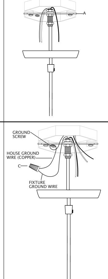
10. Slightly loosen ground screw on mounting bracket (A). Do not completely remove ground screw. Wrap ground wire from junction box around ground screw, leaving enough ground wire to attach to fixture ground wire. Twist end of fixture ground wire and end of house ground wire together. Twist wire nut (C) onto ends of wires. Completely tighten wire nut (C). Reference chart below for correct wire connections.
