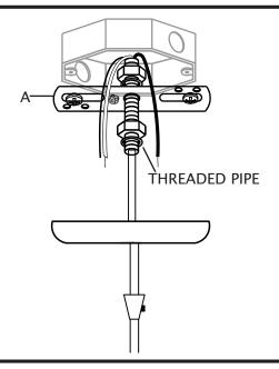
10. Slightly loosen ground screw on mounting bracket (A). Do not completely remove ground screw. Wrap house ground wire (copper) around ground screw, leaving enough ground wire to attach to fixture ground wire. Twist end of fixture ground wire and end of house ground wire (copper) together. Twist wire nut (C) onto ends of wires. Completely tighten wire nut (C). Reference chart below for correct wire connections.
