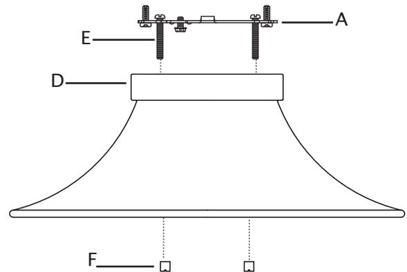
12. Screw recommended bulb (E26 Edison bulb type, not included) into socket. Verify correct bulb wattage marked on socket of fixture. **WARNING: DO NOT** exceed maximum bulb wattage.
