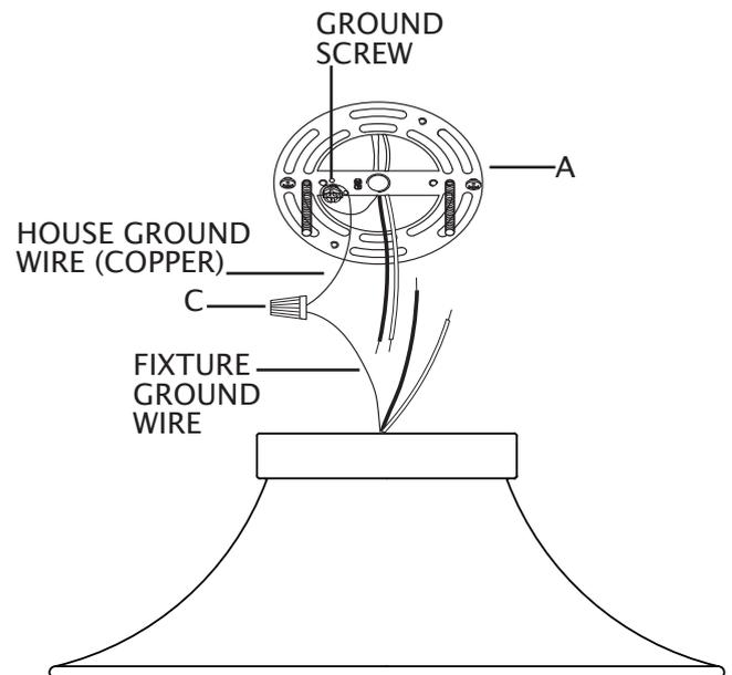
7. Twist end of house lead wire (black) and end of fixture lead wire together. Twist wire nut (C) onto ends of wires. Completely tighten wire nut (C). Twist end of house neutral wire (white) and end of fixture neutral wire together. Twist wire nut (C) onto ends of wires. Completely tighten wire nut (C). Reference chart to the right for correct wire connections.
