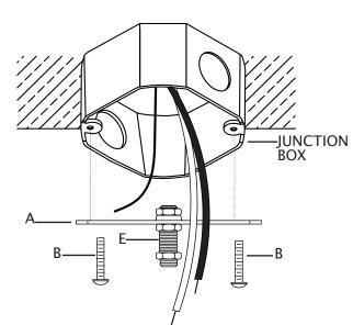
**IMPORTANT**: The length of the cord must be adjusted before fixture is installed.
