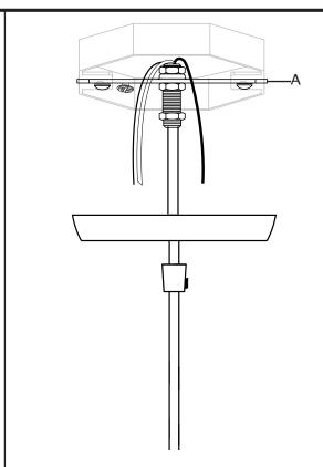
10. Slightly loosen ground screw on mounting bracket (A). Do not completely remove ground screw. Wrap ground wire from junction box around ground screw, leaving enough ground wire to attach to fixture ground wire. Twist end of fixture ground wire and end of house ground wire together. Twist wire nut (C) onto ends of wires. Completely tighten wire nut (C). Reference chart below for correct wire connections.
