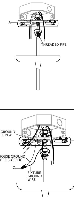
11. Slightly loosen ground screw on mounting bracket (A). Do not completely remove ground screw. Wrap house ground wire (copper) around ground screw, leaving enough ground wire to attach to fixture ground wire. Twist end of fixture ground wire and end of house ground wire (copper) together. Twist wire nut (C) onto ends of wires. Completely tighten wire nut (C). Reference chart below for correct wiring instructions.
