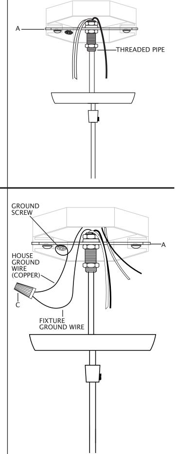
10. Slightly loosen ground screw on mounting bracket (A). Do not completely remove ground screw. Wrap house ground wire (copper) around ground screw, leaving enough ground wire to attach to fixture ground wire. Twist end of fixture ground wire and end of house ground wire (copper) together. Twist wire nut (C) onto ends of wires. Completely tighten wire nut (C). Reference chart below for correct wire connections.
