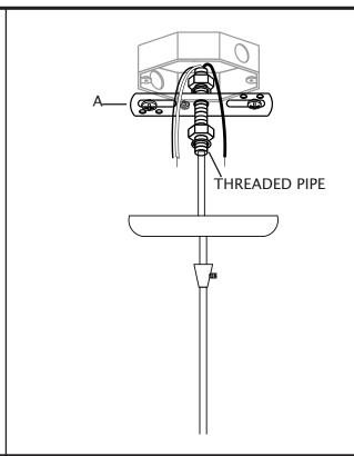
10. Slightly loosen ground screw on mounting bracket (A). Do not completely remove ground screw. Wrap house ground wire (copper) around ground screw, leaving enough ground wire to attach to fixture ground wire. Twist end of fixture ground wire and end of house ground wire (copper) together. Twist wire nut (C) onto ends of wires. Completely tighten wire nut (C). Reference chart below for correct wire connections.
